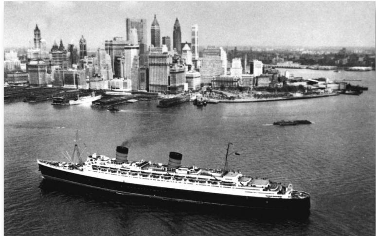
So, let’s think like Fuller of a ship the size of the *Queen Elizabeth*. The rudder of the *Queen Elizabeth* weighed a staggering 140 tons. That’s just the rudder. The force needed to push that massive rudder to the left or the right would have required hydraulic engines that would have been massive.
